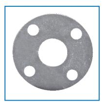
Style 8137M is a compressed non-asbestos sheet gasket material produced from aramid fibers, reinforced with a woven wire mesh and bonded with a nitrile rubber (NBR). The sheet has a graphite surface treatment for anti-stick purpose. An ideal gasket material suitable for applications with fluctuating pressures and temperatures. 8137M has a broad range of applications in the process industries and in the water and wastewater industry. Commonly used in equipment such as pumps and valves.
